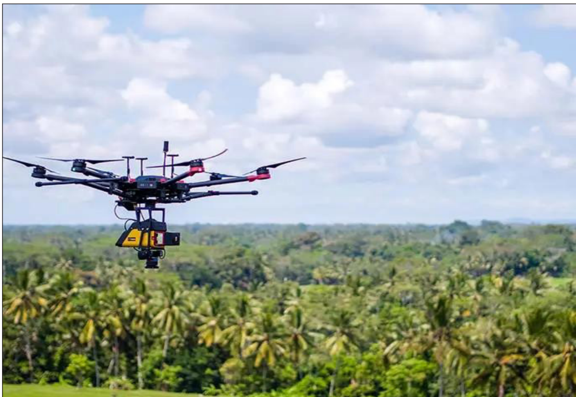
Figure 4. Drone equipped with a LiDAR and camera payload conducting aerial survey operations over agricultural and forested landscapes 8
