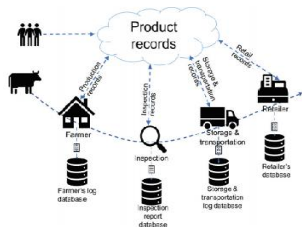
Figure 2. Cold chain traceability system
