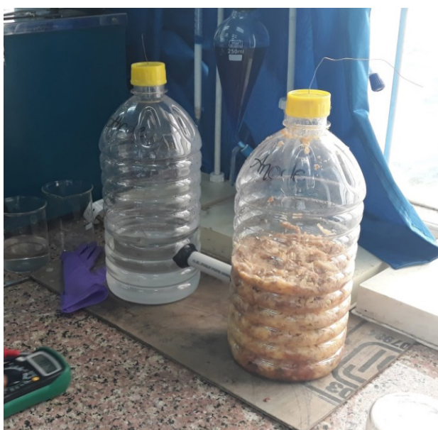
Figure 1. Setup of Microbial Fuel Cell.
