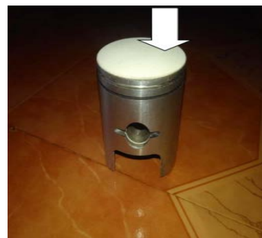
Figure 1(b).Piston after coating
