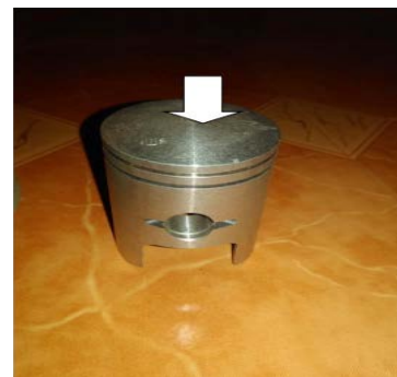
Figure 1(a).Piston before coating
