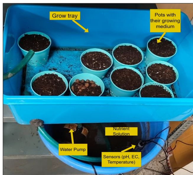
Figure 2. Experimental Ebb and Flow hydroponic system showing reservoir, grow tray, and piping. The cyclic flood and drain cycle ensures oxygenated roots and nutrient distribution, a critical feature supporting system efficacy
