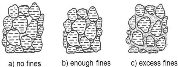
Figure 1. Physical state of soil- Aggregate Mixes (Yoder, 1975)
