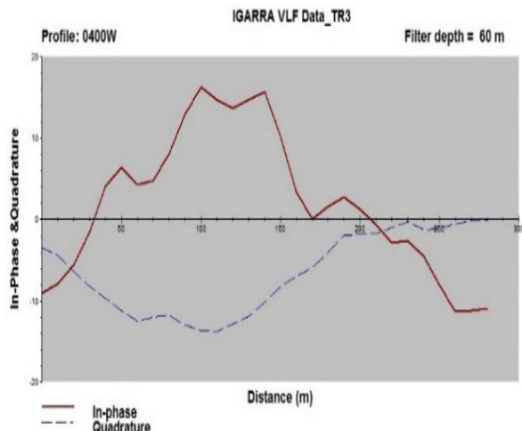
Figure 10(b).karous & Hjelt Filterrr for traverse 3
