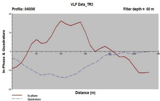
Figure 9(b).Karous & Hjelt filter fir traverse 2
