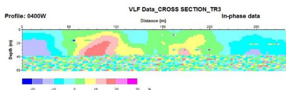
Figure 10(c).karous & Hjelt Filterrr for traverse 3
