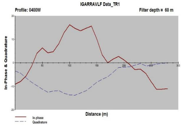
Figure 8(b).Karous & Hjelt filter for traverse 1
