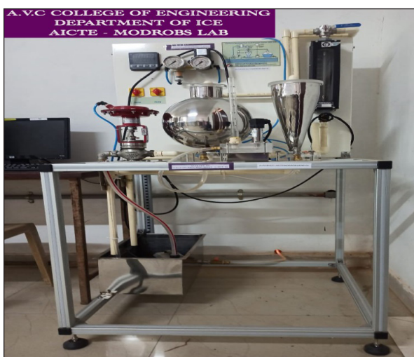
Figure 1. Labeled Photograph of The Conical & Spherical Tank Level Process Trainer
